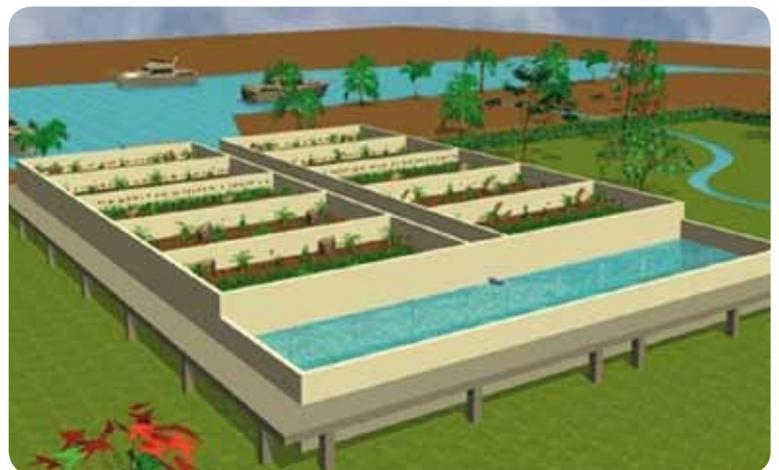
in this type of system. No chemical products are needed. The water is treated in three weeks. Some is used to irrigate crops and some is emptied back into the lake. The dried faecal sludge is sold as fertiliser, and the purifying plants are used as fodder for livestock.
